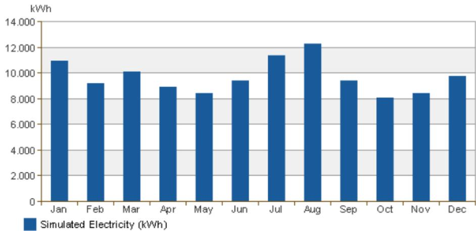
Figure 4. The monthly electricity consumption over the year
