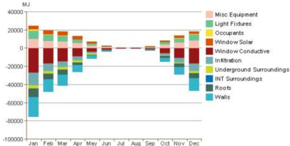
Figure 3. The monthly heating load of the building over the year
