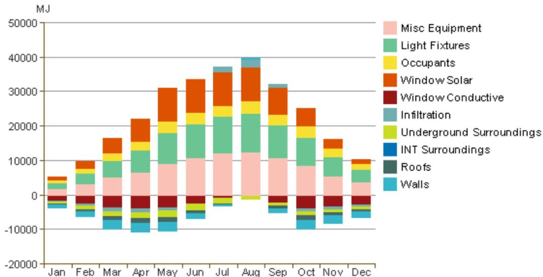
Figure 2. The monthly cooling load of the building over the year
