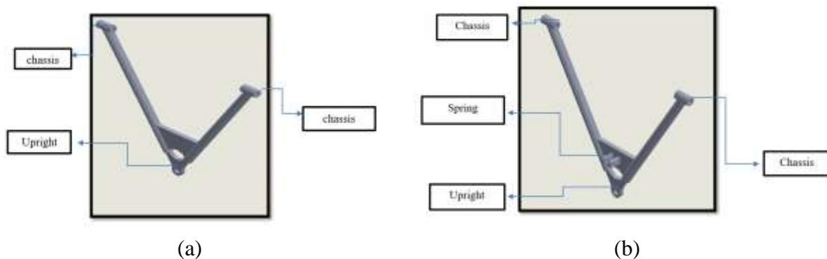
Figure 1. Design of the suspension arms (a) upper arm, and (b) lower arm
