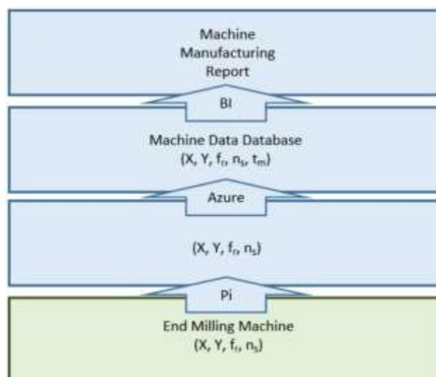
Figure 1. Flow chart of the prototype
