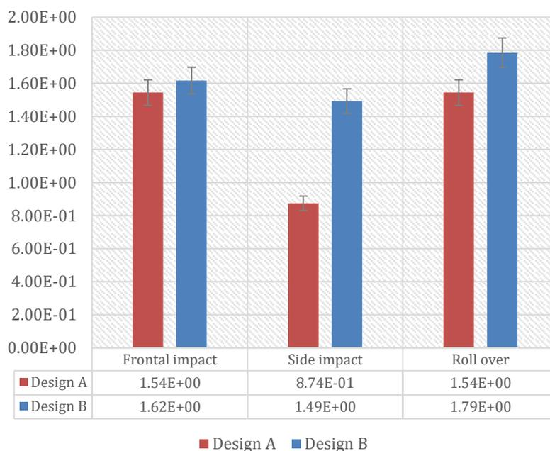
Figure 1. Comparison of factor of safety against the impact test on design A and B.
