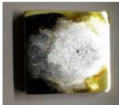
Figure 3. Surface condition of AISI 304 alloy steel after nitriding.
