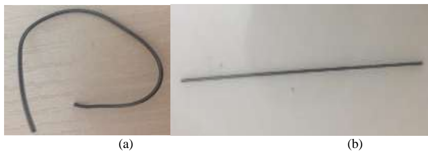
Figure 1. (a) The deformed shape in martensite phase, (b) Recovered shape in austenite phase
