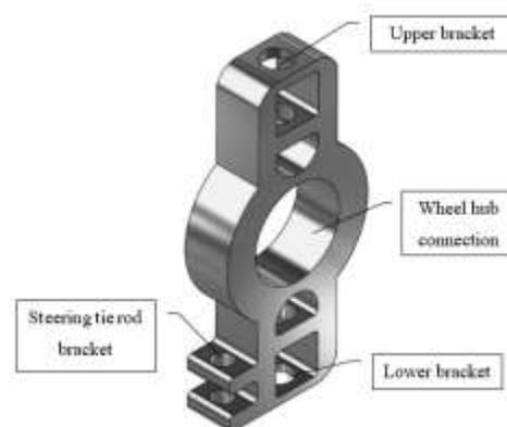
Figure 1. Design of the upright structure
