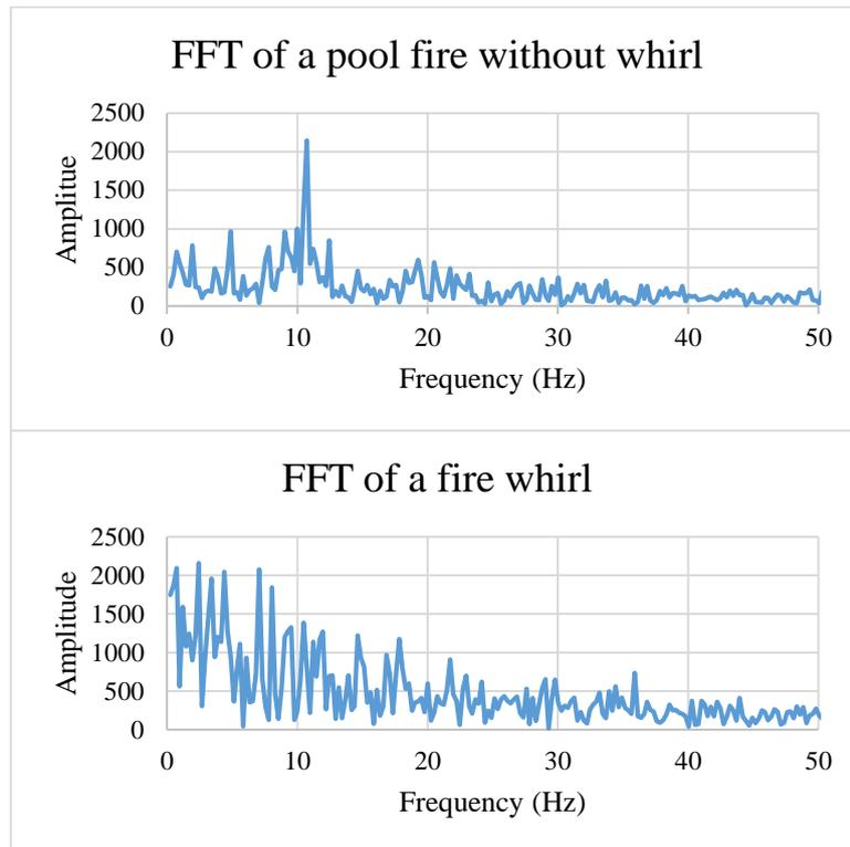
Figure 4. Frequencies of a small-pan fire (top) and a fire whirl (bottom); Fuel: Ethanol
