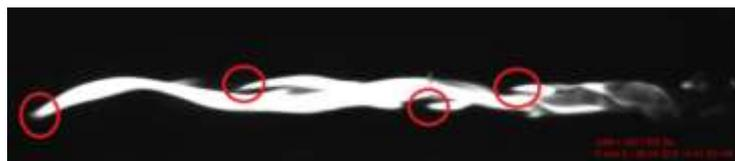
Figure 5. Multiple peaks of fire whirls (Top is on the left; gravity to the right)
