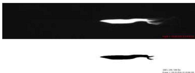
Figure 2. Sample fire image conversion (top: original, bottom: processed)
