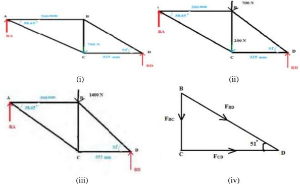
**Figure 1.** (i) Static start-up, (ii) Steady pedalling (iii) Vertical loading, and (iv) Rear wheel braking
