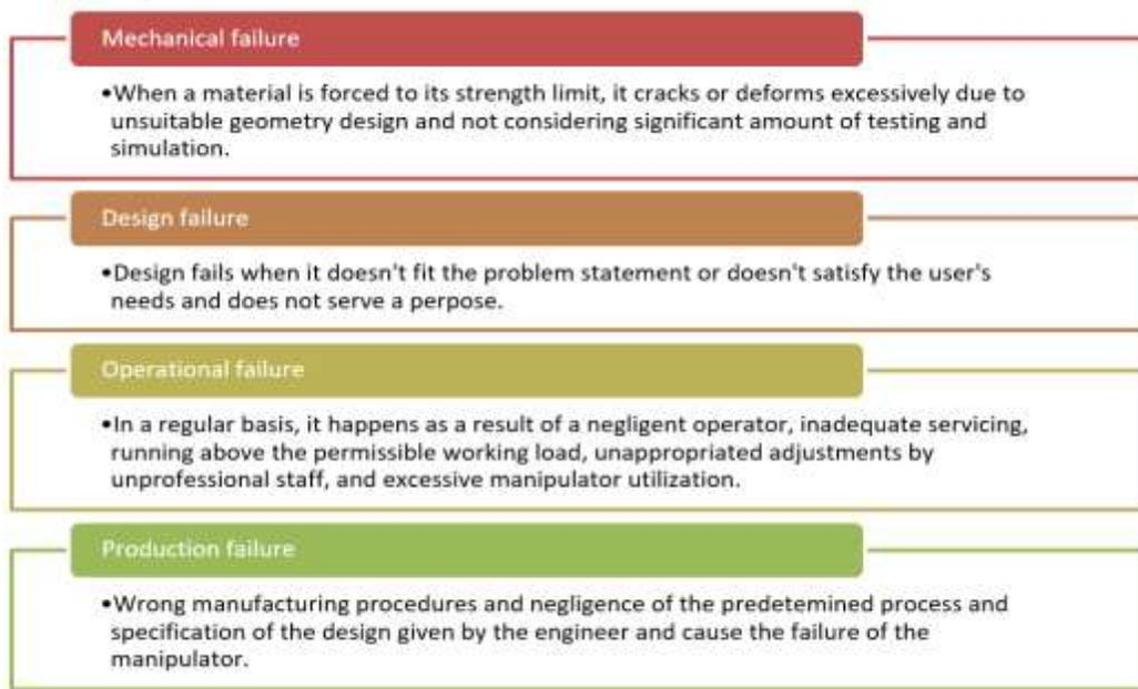
**Figure 5.** Industrial manipulator failures
