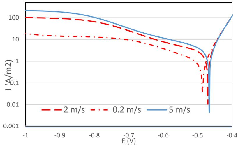
**Figure 5.** Effects of water flow rate at condition: 1 bar, 2 % CO<sub>2</sub>, 10% H<sub>2</sub>S, pH 4, 40°C. as calculated based on electrochemical theories.
