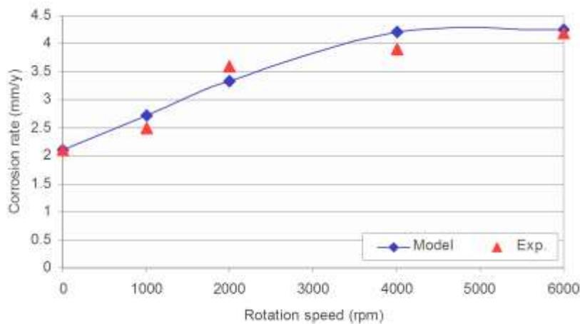
**Figure 7.** Effect of rotation speed on corrosion rate; a comparison between model and Martin's experiments (saturated CO<sub>2</sub> solutions, 40 ppm HAc, pH 6, and Temperature 60°C ).
