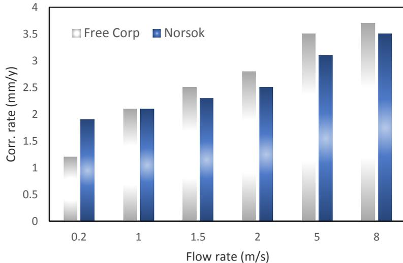
**Figure 4.** Comparison of effects of flow rate on corrosion rate calculated by Norsok and Freecorp.
