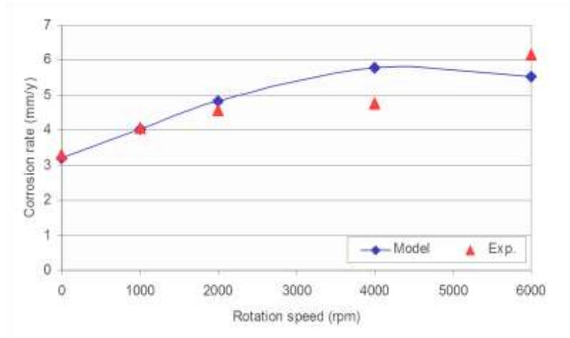
**Figure 6.** Effect of rotation speed on corrosion rate; a comparison between model and Martin's experiments (saturated CO<sub>2</sub> solutions, 60°C, 20 ppm HAc, and pH 5).
