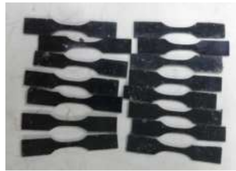
Figure 1. ASTM D1822L test specimen size
