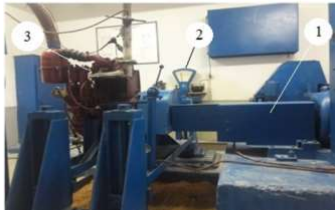
Figure 3. D-21A1 engine of test stand KI-5343M general appearance (1-KI-5543M test stand; 2-PSID - electronic scale; 3-D-21A1 engine)
