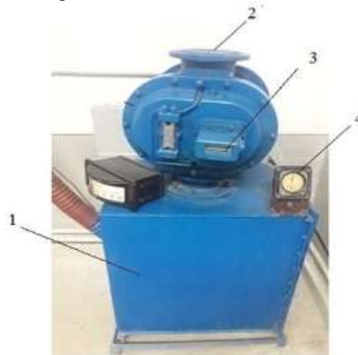
Figure 6. Air consumption meter RG-200 (1 receiver; 2nd air cleaner; 3-air consumption meter; 4th stopwatch)
