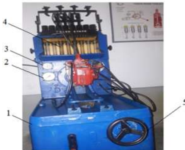
Figure 1. KI 921 control test stand (1st base; 2-manometer; 3-tachometer; 4-measuring beakers; 5- screw adjusting the rotation speed of the drive shaft)
