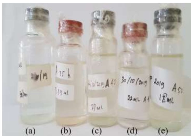
Figure 1. Reflux Results a) 30 hours; b) 35 hours; c) 40 hours; d) 45 hours; and e) 50 hours
