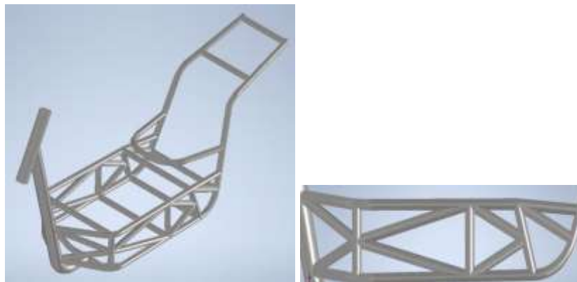
Figure 7. Isometric and side view of chassis design 5.
