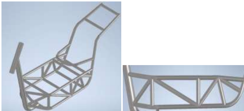
Figure 3. Isometric and side view of chassis design 1.
