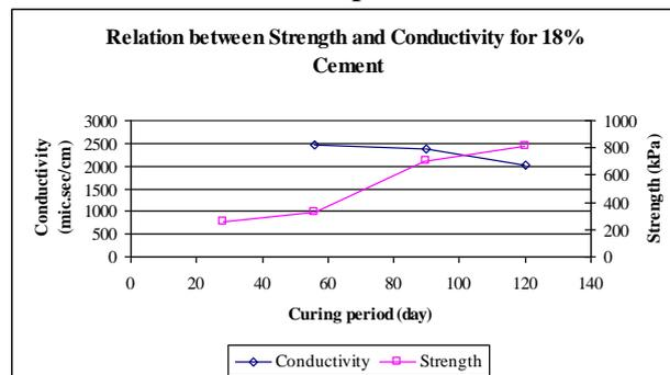
**Figure 10.** Relationship between Strength Development and Ionic Conductivity for 18% Samples
