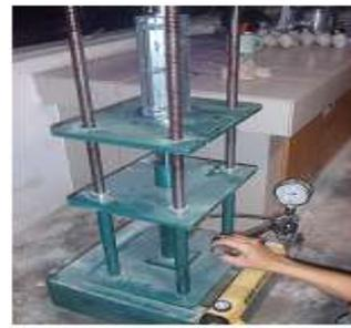
The static packing pressure apparatus
