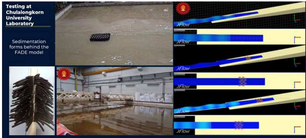
Figure 3. Laboratory testing and CFD simulation of FADS
